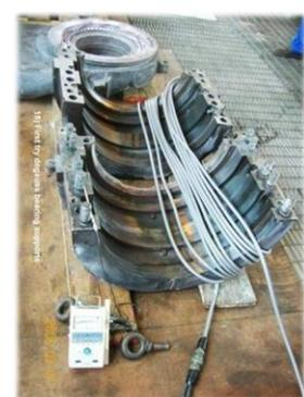
Measuring tools for control of degaussing
