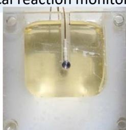
Monitoring polymerization by ultrasonic method
