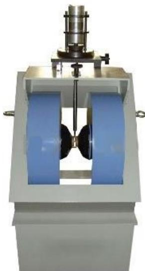
Low gap electromagnet for high field calibration (> 2 Tesla)
