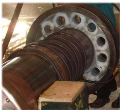
Complete degaussing of massive parts
