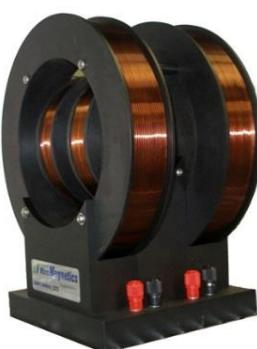
Helmholtz assembly for 1-axis measurement calibration
