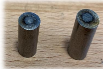
Fe-C steel samples analyzed by spark spectrometry
