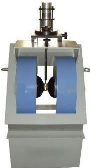
Low gap electromagnet for high field calibration (> 2 Tesla)
