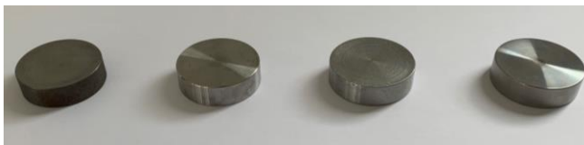
Shims of different steels and cast irons with known magnetic permeability
