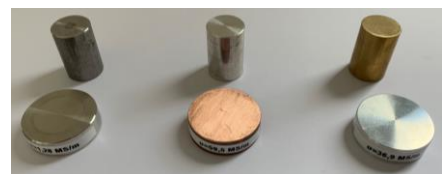
Shims of different conductive materials with known electrical conductivity
