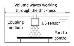
US sensors in film form working in surface waves and in thickness
