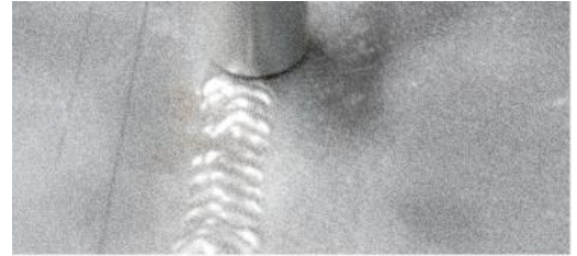
Measurement of the ferrite rate and the evolution of \mu_r on the weld bead
